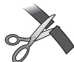
If necessary, remove the malleable metal stay and bend it to the appropriate position.
